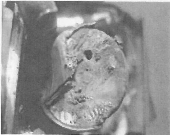
Figure 7. MOV failure caused by thermal runaway and internal equipment fire in a surge protective device.
