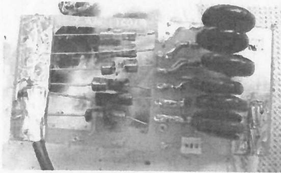
Figure 14. Six parallel arrangements of 3-amp, slow-blow fuses in series with 510 volt MOVs on a test card after one 1.71 p.u. (473.4 V<sub>rms</sub>) 64-cycle duration TOV: four out of six fuses blown with three out of six MOVs damaged (epoxy surfaces lifted).
