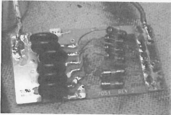
Figure 16. Six parallel arrangements of 3-amp, slow-blow fuses in series with 510-volt MOVs on a test card after 39 5.5-kV surges: five out of six fuses blown with no MOV damage.
